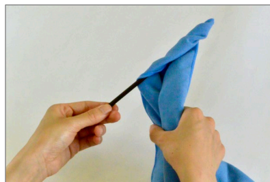
C. Thread the cloth to the cleaning rod D. Wrap a cloth around the cleaning rod E. Wipe the water inside the recorder
