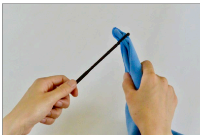
C. Thread the cloth to the cleaning rod D. Wrap a cloth around the cleaning rod E. Wipe the water inside the recorder
